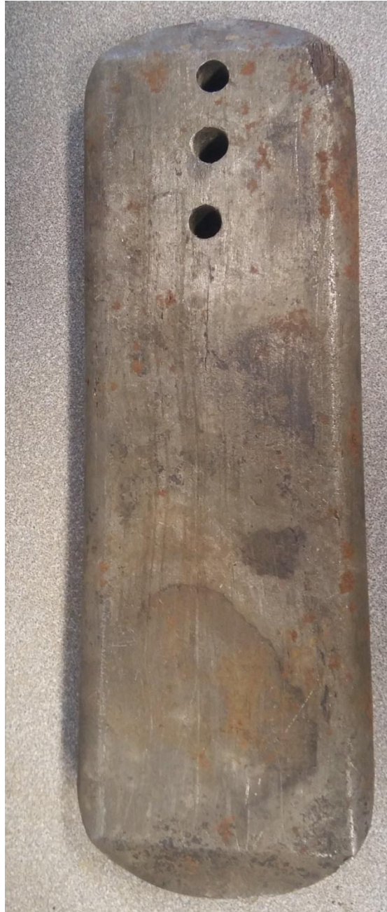
Fig 4: Mechanical Key recovered from the flywheel pit.
