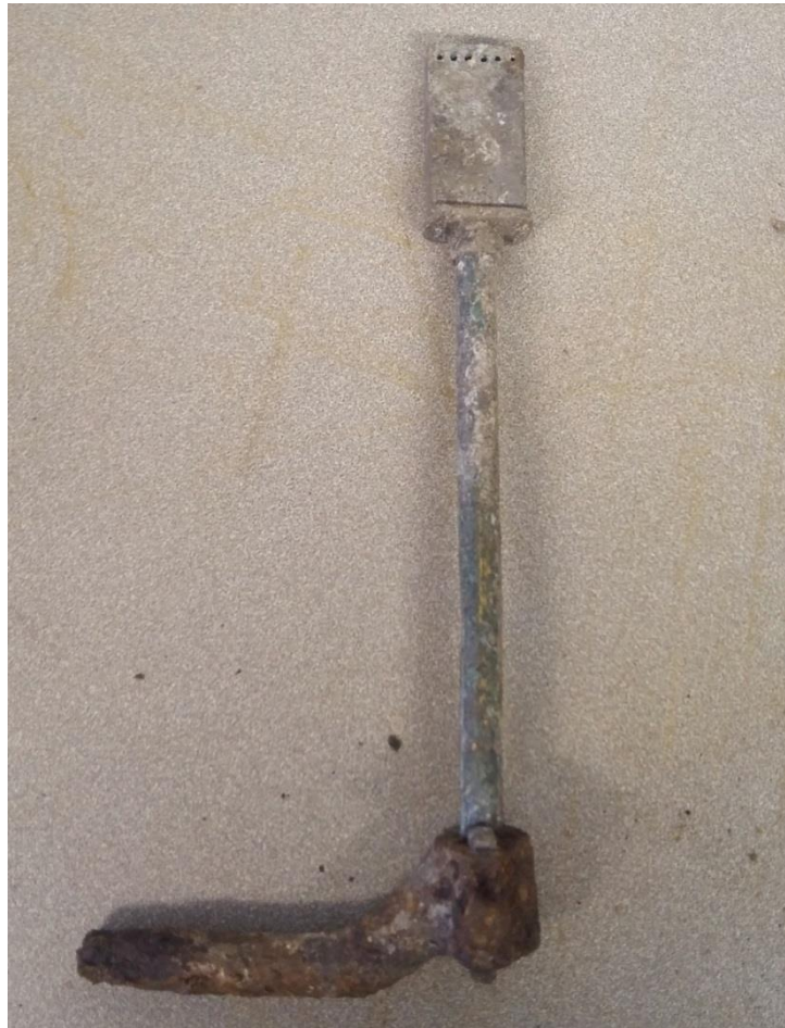
Fig 6: Image of the larger cotton burner, used in the gassing stages of yarn production
