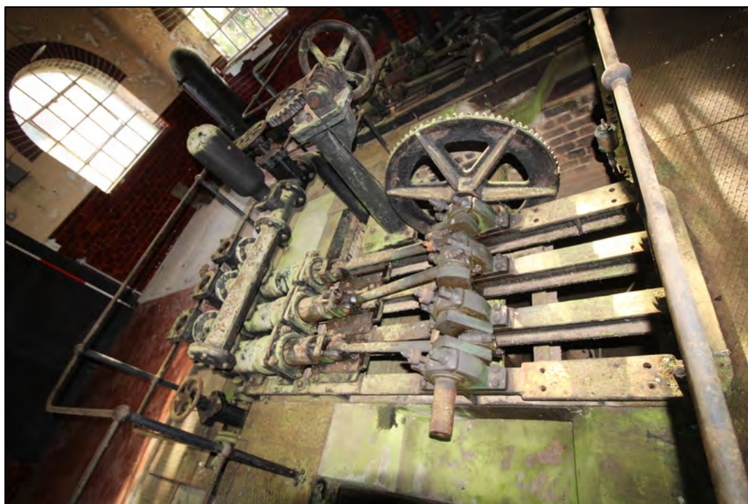
Plate 28: Crankshaft bearing bolts, crankshaft and pistons of central turbine pump
