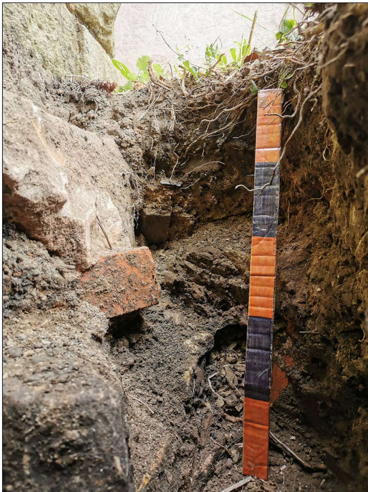
Plate 8: View of Trial Pit 1 showing stone and brick rubble, looking east
