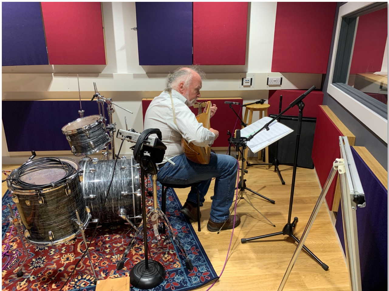
Figure 5 11 - A photograph of the recording taken in the booth in Studio 1 at Salford University, used to attempt a clean capture using a combination of an AKG C414 microphone for the body and a Schoepps pencil microphone for the neck of the instrument
