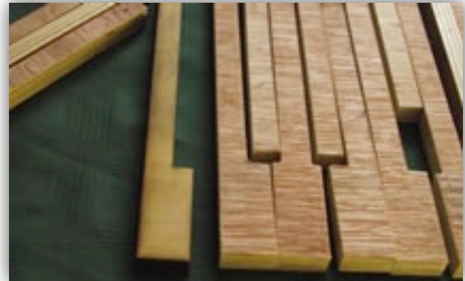
Outputs from CNC and laser cutter compared (Brissenden P. G., Reverse Action Piano Harp, 2013)
