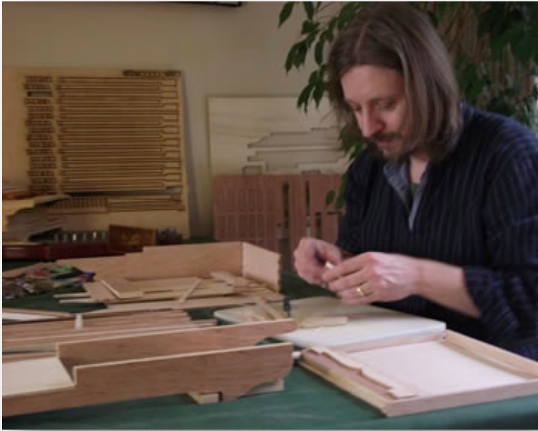
Trimming and sanding the output from CNC and laser cutter (Brissenden P. G., 2012)
