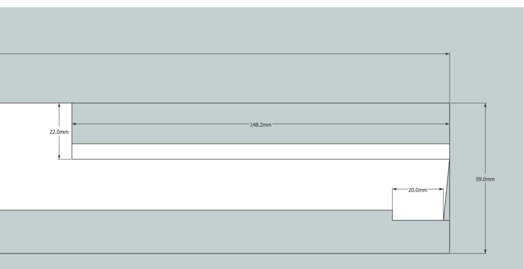
Shows the enlarged detailed measurements moving clockwise around the block The angle of cutaway is another 84.3°.
