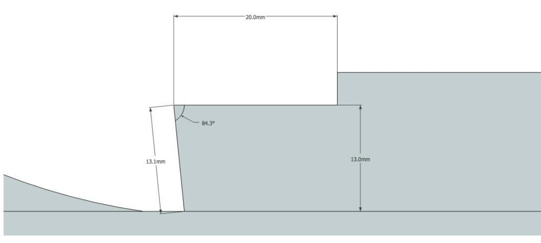
A 3d projection showing the finished cross spar. Curved edges will be smoothed.
