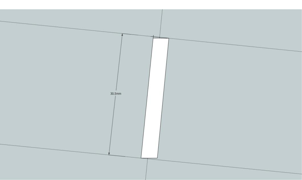
The Toe Cross Spar is shown here with 1.11 Lid Side Arm. This is because both can be generated from the same block. I suggest a starting block which allows a slight cutting margin on 466x59x12mm.
