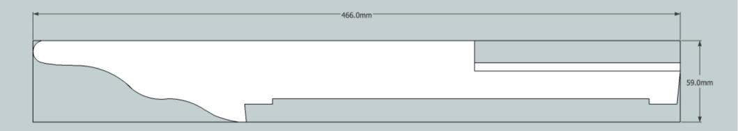
Execute the first cutaway at the top of the block, and put the smaller block aside to fabricate 1.11 Lid Side Arm.
