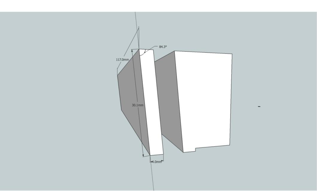
**1.2 Comb Backing** End enlarged from a 2d projection – shows the very slight cutaway needed.
