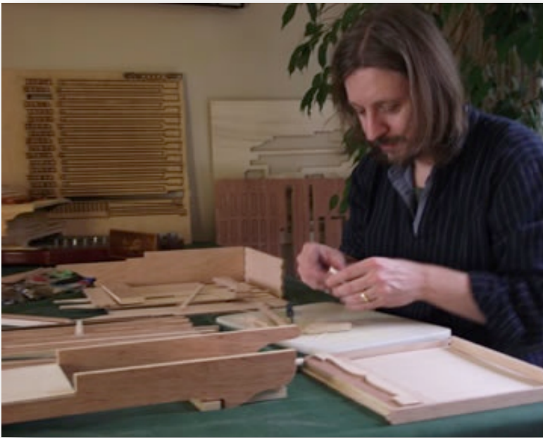
Figure 16. Trimming and sanding the output from CNC and laser cutter (Brissenden P. G., 2012)
