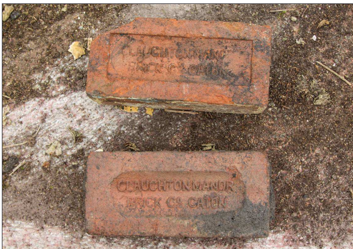
Plate 16: Two types of machine-made, froged bricks found in the demolition rubble, likely associated with the footwear factory
