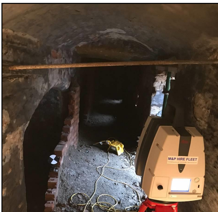
Plate 10: View of the corridor taken during the laser scanning
