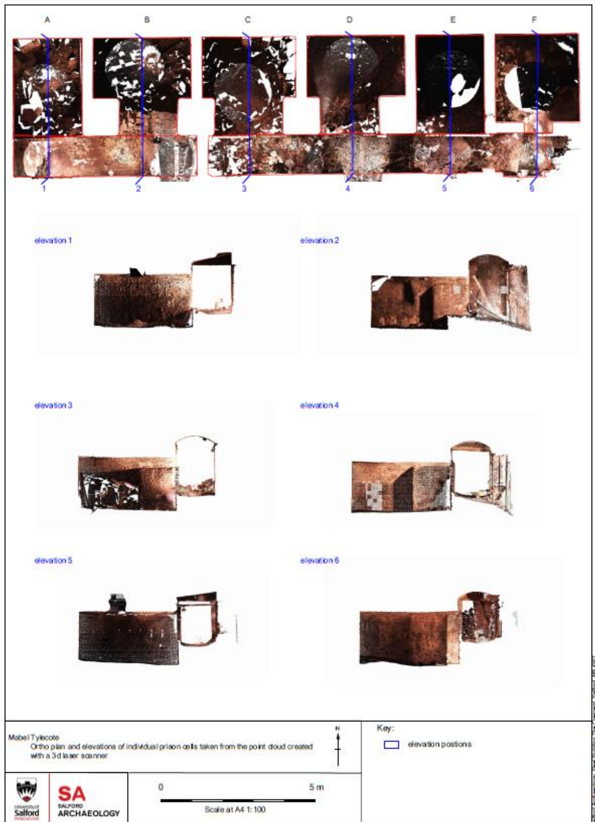
Figure 5: Orthographic plan and elevations produced from the laser scan results
