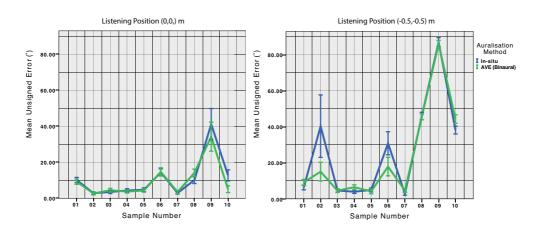
**Figure 2.** The mean unsigned error for in-situ and AVE auralisation methods at listening positions (0,0)m and (-0.5,-0.5)m across all subjects.
