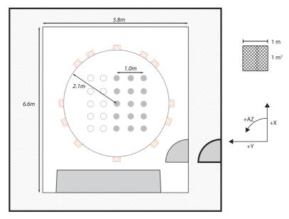
Figure 1. Plan view of the measurement setup and coordinate system used in the dataset.
