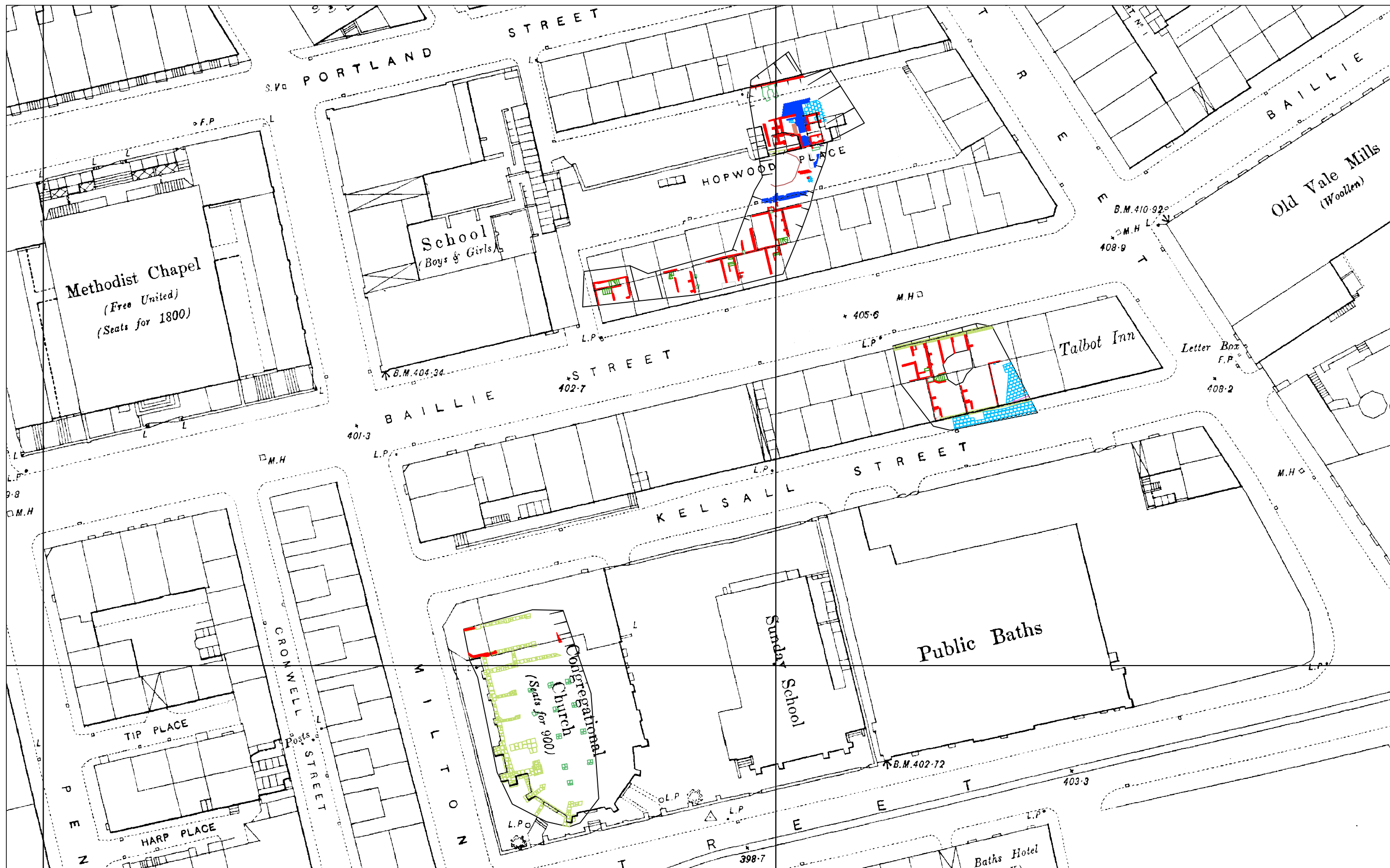
Figure 14: Excavation Plans Superimposed onto 1892 OS 1:1500 Town Plan
